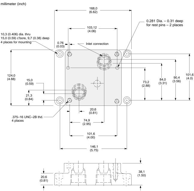
NOTE: When the subplate is not used, a machined pad, as indicated by the shaded area on the subplate, must be provided for mounting. The pad must be flat within 0.0127mm (0.0005 inch) and smooth within 63 microinch. Mounting bolts, when provided by the customer, must be SAE grade 7 or better.
