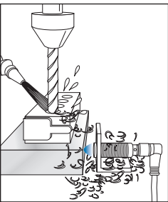
Ferrous-only technology ignores aluminum chips and eliminates false signals.
