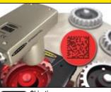
Objective: To detect and verify a dot-peened bar code on a metal part. page 370
