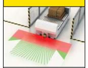
Objective: To detect the presence of personnel or objects in the path of the automated guided vehicle (AGV).
