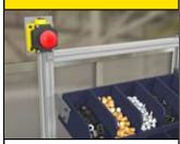
Objective: To alert personal to refill bins before parts are depleted.
