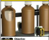
To detect water or liquid containing water, regardless of bottle color.
