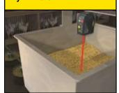
Objective: To accurately determine the level of dry bulk material in a bin hopper, despite the material's uneven surface.
