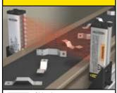
Objective: To accurately detect flat objects passing on a conveyor.
