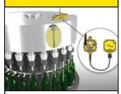
Objective: To monitor fill level, temperature and pressure to determine when to activate the inflow into the tank
