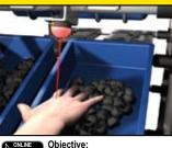
To indicate whether the operator is picking from the correct bin or page 444 wrong bin.
